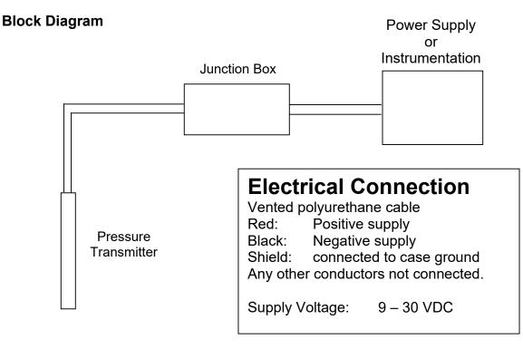
Inside the Junction box will be the surge protection which will be have the "IN" terminals label 1 & 2 and the OUT terminals labeled 3 & 4. Connect the device so that the "IN" points in the direction from which the surge is expected (the field wire). Connect the "OUT" terminals (3 & 4) to the Pressure Transmitter wires. Terminal 1 on the "IN" corresponds to terminal 3 on the "OUT" and terminal 2 on the "IN" corresponds to terminal 4 on the "OUT". Polarity does not matter on this device.
