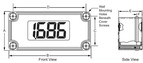
A: 80mm (3.15") C: 60mm (2.36") E: 65mm (2.56") B: 140mm (5.51") D: 120mm (4.72") F: 20mm (.79")
