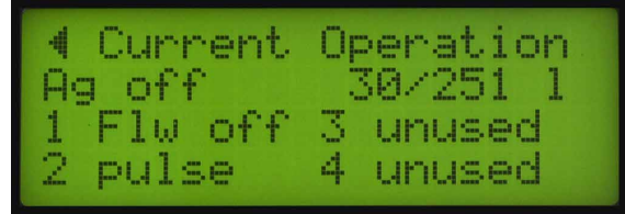
Current Operation Screen with 30 liters of water to be treated and more water needed to reach the 251 liter minimum to run for 2 minutes
